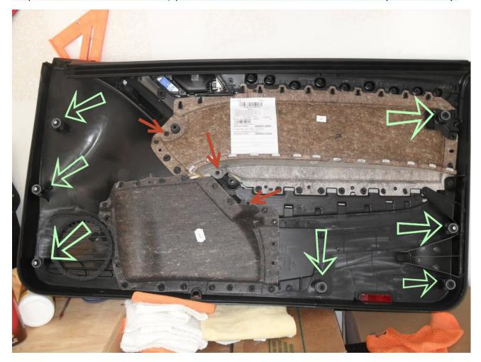
Step 5: Remove the door handle, you will need to unscrew 3 T15 torx screws (shown in red):
