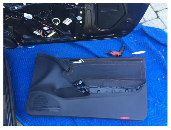
Step 2: Start by applying glue going from top to bottom, first door insert. Glue the main part of the door panel insert first. Then use the pry tool to stick the stitching between the door insert and armrest. After that glue the armrest main part. Wait until the glue is dry, and then glue the sides.
