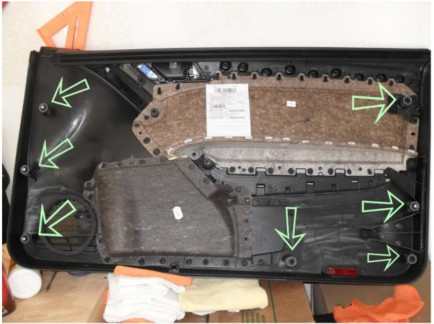
Start with lower rear corner (bottom right in this pic) then slide your hands under the panel and slowly move towards the front of the car while slightly pulling towards my body. Try not to lift or pull down on the panel, but pull as straight outward as possible. Once you have unclipped to the three along the bottom move up along sides remembering to pull straight out.
