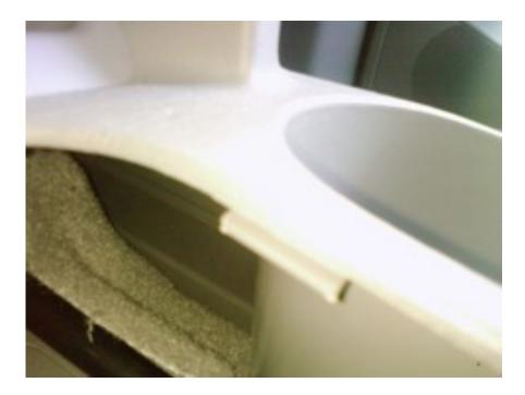
If your shift boot has a trim piece on top, you need to transfer it over to the new boot. Remove it from the stock boot and install it into the collar of our boot, like so. It can be done with a wax cord, or zip-tie, whichever is more available to you.
