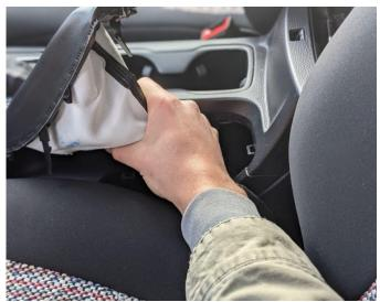
3. Remove the e-brake boot from the retaining ring by slipping a thin object between the boot and the ring. The glue is very easy to split.
