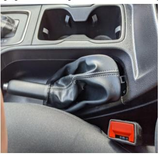
2. With the retaining ring released pull the ring out so the boot is turned inside out, twist and pust the boot up off of the e-brake handle.
