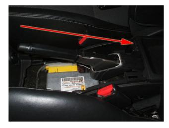
**Step 4:** Cut and discard the plastic piece on top of the e-brake mechanism using a razor knife. Use the knife to shave the raised plastic portion of the handle down until the MOMO handbrake handle fits snug. Test for snug fitment often as you shave down the plastic to ensure you don't remove too much.
