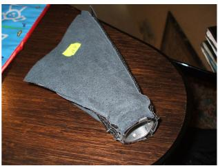
**Step 6**: Re-install the e-brake bezel and new boot / handle combo by placing the shifter knob back into 3<sup>rd</sup> gear and pulling the e-brake as high as it will extend. This will allow you to mock the bezel in position as shown and tighten the locking screws for the MOMO handle. If the leather boot is blocking the screw holes, use the razor to remove the area that is blocked. Be sure to align the boot properly before snapping the bezel back into place.
