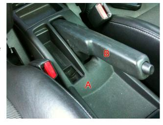
**Step 2**: Cut the e-brake handle cover as shown and discard the front portion as it will not be needed for this installation.
