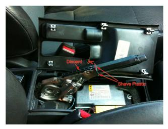
**Step 5**: Remove the black plastic retainer on the end of the e-brake handle. Invert the e-brake boot and place the e-brake handle inside of the boot as shown. Ensure that the bottom of the e-brake handle is in line with the single lower stitched line on the boot. The top of the handle should be centered between the two upper stitched lines on the boot. Use a zip tie to hold the boot firmly in place.
