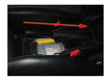
**Step 5**: Re-install the e-brake bezel by sliding it over the handle and boot and secure it by pressing down. Ensure that you hear the metal clips snap into place. *That's it!* Test that the e-brake boot doesn't snag by extending and releasing the e-brake a couple of times. Also ensure that the operation of the e-brake is not restricted. Make necessary adjustments accordingly.
