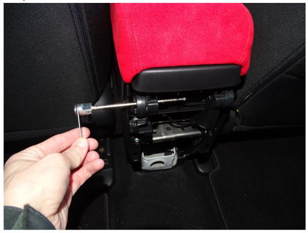
Then slide the cover and remove the 5 Phillips screws and pop the cover off and proceed with gluing the new Redline fabric to the OEM fabric.
