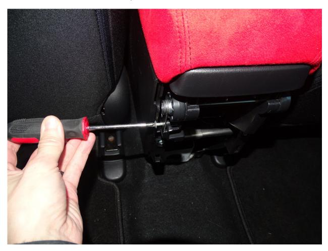
You'll then need to push the bar to the left a little bit and rotate counter clockwise and pull the rest of the way out.
