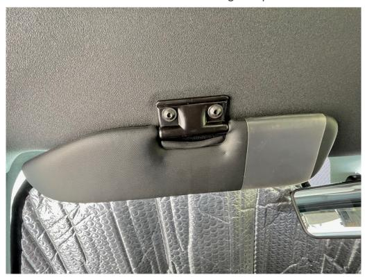
Insert the visor into the appropriate cover (each side is different). Secure the velcro and bolt the visors back into place.
