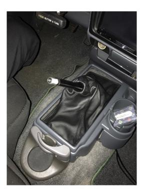
View of Cup holder not all models have this, to remove push down and slide towards rear of vehicle
