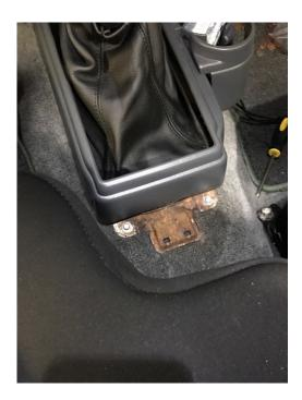
There are 4 screws holding down the center console, 5 if you have the side cup holder. Remove screws to remove console
