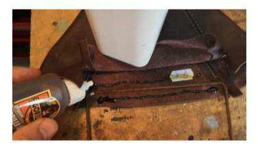
After you've applied the glue, fold the flap over the frame. Using the pieces of wood (or Popsicle sticks, or whatever you're using) on both sides of the flap, clamp the flap down.
