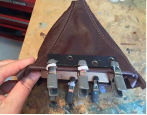
In this installation, the glue was allowed to set on the two sides of the boot before gluing down the remaining two sides, as you can see in this photo. However, that's not necessary and you can glue all
