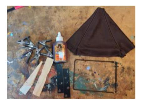
In this step, you're going to place each side of the frame over the corresponding side of the boot, then lay down glue on either side, fold the flap of the boot over the frame, and clamp it down until the glue dries.
