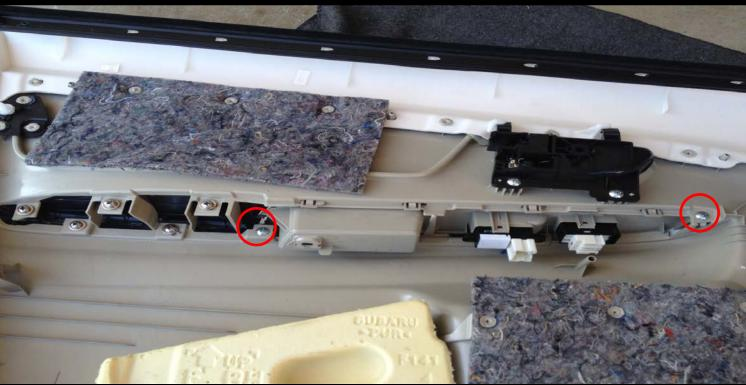
Reinstall Door Panel, Do not forget to re-attach the cables and electrical connectors.
