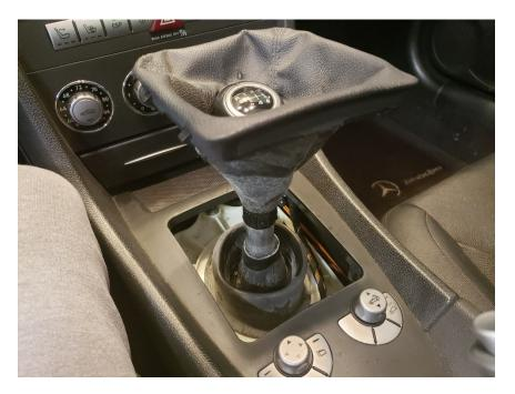
3. Rotate the plastic collar 1/16<sup>th</sup> turn counter-clockwise (when looking from the top). Then pull the collar downward.
