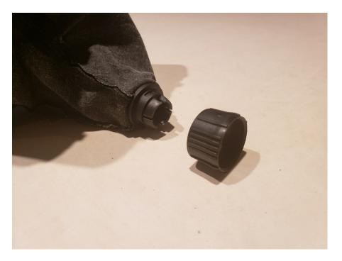
6. Pry off the boot retainer ring with a thin screw driver.
