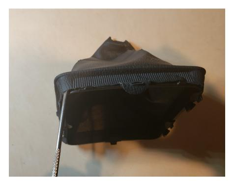
9. Trial fit the new shift boot on the plastic frame.
