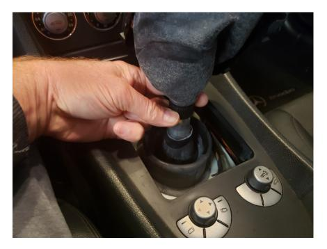
4. Pull the shift knob straight upward to remove.
