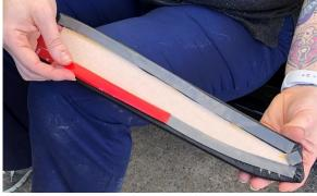
5. Align door padded armrest with factory armrest, pressing flat edge against the door and aligning the edges.
