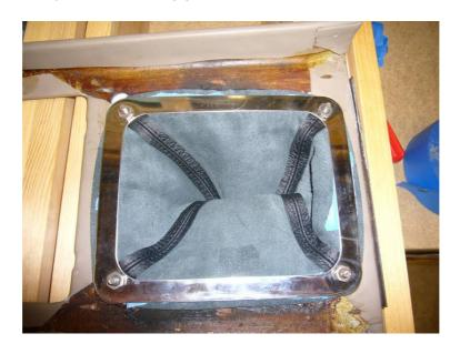
Step 7: Install the consol over the shifter. If desired you can do a reverse of the boot and fasten it to the shifter with a zip tie. (I did not do this because for shows I want to be able to quickly change to the OEM boot and it looked fine as is)
