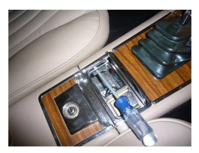
Step 3: Remove ash-tray bezel and disconnect cigarette lighter wiring
