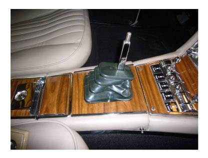
Step 2: Unscrew consol cover screws (2), remove ash tray, and unscrew ash-tray bezel screws (2)
