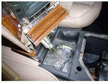
Step 4: Remove consol cover, and remove existing shifter boot trim plate and nuts (4)
