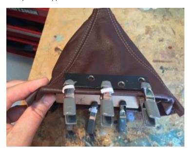
In this installation, the glue was allowed to set on the two sides of the boot before gluing down the remaining two sides, as you can see in this photo. However, that's not necessary and you can glue all four sides at the same time.
