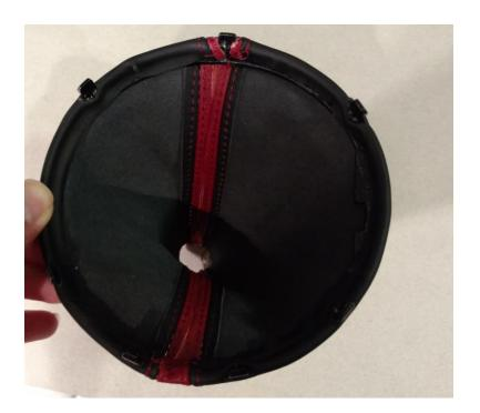
8) Now you are ready to reinstall. Depending on the materials you pick, the boot may not stretch as much as the stock material. If your boot is too tight to clear the reverse lock-out, cut a vertical slit from the top of the boot down to the point where you are able to clear the lock-out (about 1 inch). Note that once installed, this slit will be completely hidden (but be careful cutting it, start small and enlarge if necessary).
