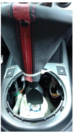
10) Turn the boot right-side out and snap the trim ring into the center console. Test shifter operation to ensure the boot is not too tight or loose. Make adjustments as necessary.
