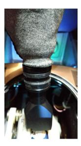
4) Return the shift boot back to its regular orientation (inside in). Peel the leather away from the the plastic trim ring on the inside bottom. Then pull the leather over the plastic prongs. This will separate the stock boot from the trim ring. You are now ready to install the new boot.
