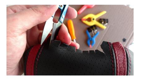
11) Secure the four corner flaps. Depending on thickness, you may need to trim these so the cover fits back on the console.
