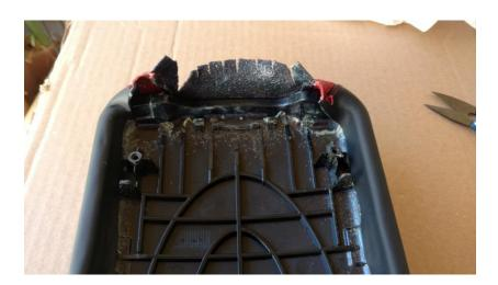
10) Repeat steps 8 and 9 for all four sides. For the front, you may need to make deeper cuts so the leather lays properly over the latch curve.
