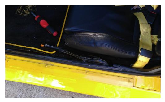
Mine have had some wear so I had to add additional screws to keep the trim panels in place. Most Fiero owners can get away with removing the front trim panel only that goes around the e-brake.
