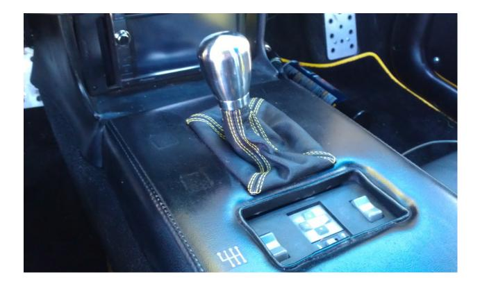
Admire your work and enjoy your new leather shifter boot. The automatic transmission shifter boot is a different cut, but the removal and installation procedure is the same for Fiero owners with the stock center console and automatic transmission.
