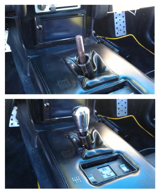
On the stock center console there are retaining screws located under the ash trays on both driver and passenger side. Once removed you will be able to lift up the shifter console. On my application my unit was all one piece. Once you have the console out remove the retaining screws from the underside holding the shifter boot in place and remove your old shifter boot.
