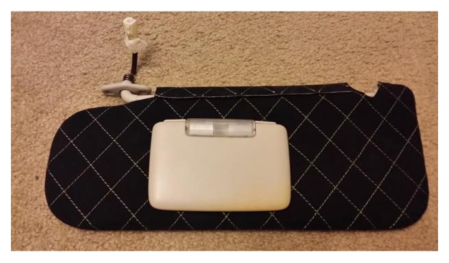
Install the mirror, don't forget to plug the light back in!
