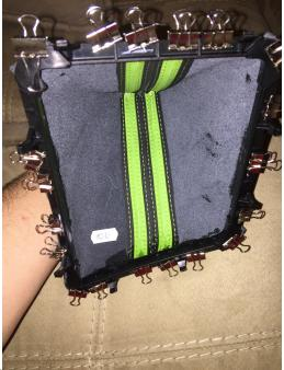
7. Once adhesive cured for 24 hours, you then simply snap the black support ring assembly into the chrome bezel trim piece, and install into center console, ensuring all black tabs are locked into bezel piece.
