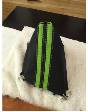
5. Once adhesive is cured around all corners, gently peel up every edge of all four sides and apply a generous (but placed carefully) amount of adhesive. I decided to ensure proper adhesion along the entire edge to use a small ruler held in place with quick clamps, as seen in photograph. I repeated this for all four sides until all sides were tacky.
