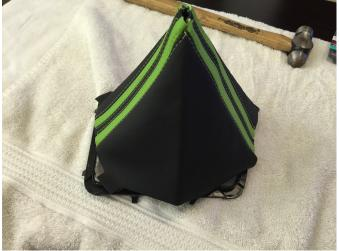
3. Lightly stretch boot over black support ring, ensuring that the tabs line up with the corner tabs as shown in image.
