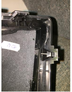
8. Here is the assembly prior to locking the tabs into the bezel.
