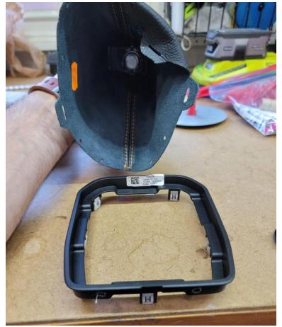
14. Replace boot. Before you forcefully click the 4 posts on the plastic frame back into the console make sure that the leather of the boot is tucked close to the plastic of the frame all the way around so that none of it bulges out. Then replace the spring.
