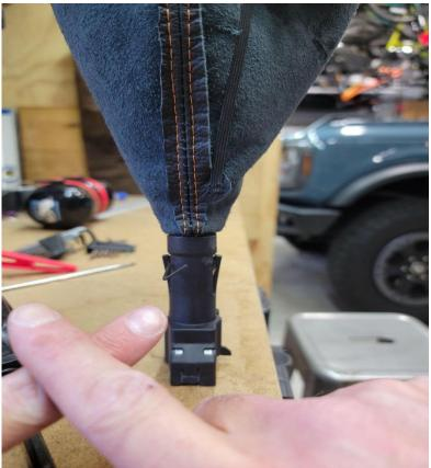
13. Attach leather replacement boot to plastic frame. Note orientation. The holes in the RedlineGoods boot are useful in case you want to further strengthen the bond by applying glue, or hot-gluing the boot to the frame.
