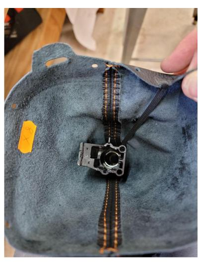
Incorrect orientation – another example. Note different orientation of stitching to long side of rectangular plastic base.
