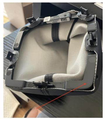
6. Remove the original shift boot fabric from the plastic frame. Before doing this look very carefully at the orientation of the boot to the black plastic sheath that goes back over the shift. This is not symmetrical, take note. I will show this again later as I made an error twice when I was installing the replacement shift boot.
