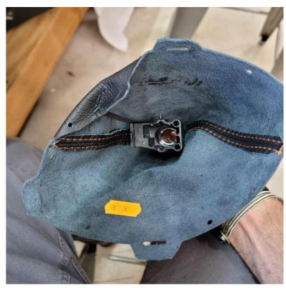
Correct orientation of stitching and elastic tensioner to plastic shifter sheath.
