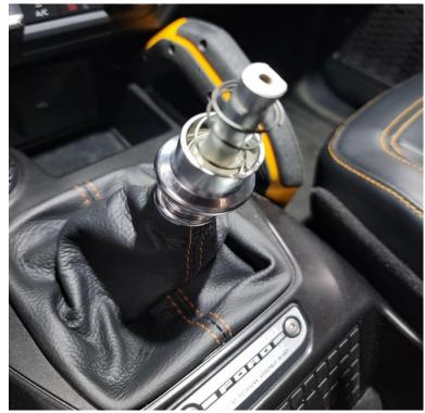
15. Replace the knob, Allen screw to secure it, and the plastic knob cap.
