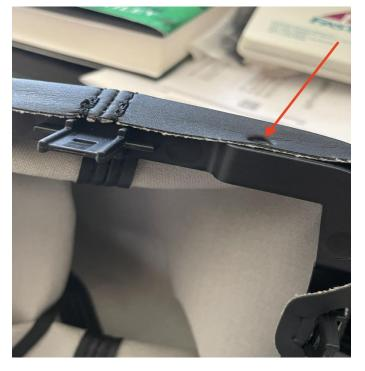
7. To remove the fabric and install the replacement you need to remove the black plastic from the metal post beneath. Get a large flat head screwdriver and carefully pull back the plastic tongues that hold this part in place. Since you can't do both sides together easily and you don't want to pull too hard, use something (like two small Allen wrench keys) to wedge plastic tongues to hold open.
