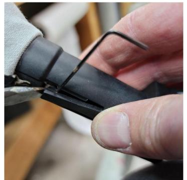
8. Separate the factory boot, the inner plastic part, and the outside metal one. Insert the metal part into the collar of the RedlineGoods Bronco shift boot. Before completing the next steps, you will want to read ahead and make sure NOW that the orientation of the plastic sheath that you are about to reinstall over the metal tube is correct in relation to the stitching of the boot, the elastic tensioner, and the asymmetry of the shift boot.
