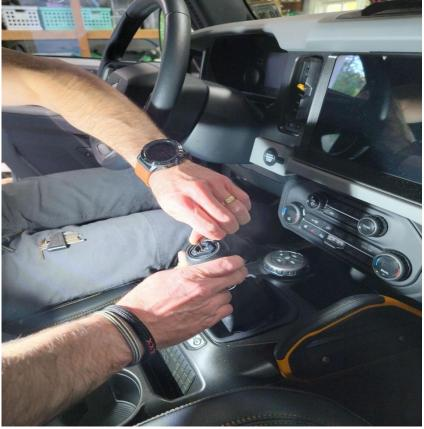
3. Remove shift knob, then remove spring and nylon spacer (all one piece)
