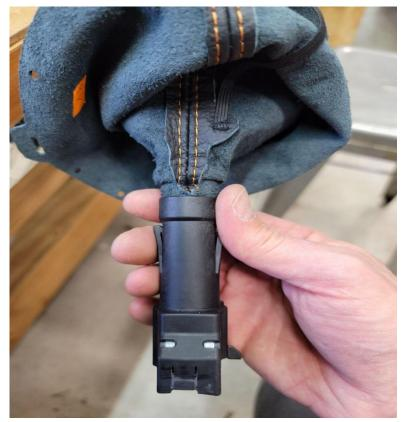
11. To force the leather to fit inside the plastic sheath I used the handle of a hammer and then tapped the hammer with a rubber mallet. Once you see the plastic tongues seat themselves back into the notches in the metal tube you are done with this step and can pull the leather down.
