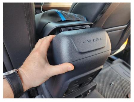
2. Open the arm rest. Use fingers or small flat head screwdriver to pry out center pin that holds the armrest to the console. (Pull all the way out). Remove armrest.
