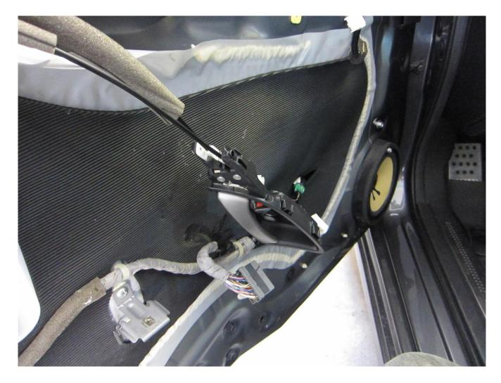
8. From here the door can be closed, no need to worry about the handle and it's cable, let it hang in place and move onto disassembly of the door panel.
