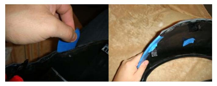
4. Allow the glue to cure and remove the tape. You should have a cleanly mounted leather cover with no air bubbles. The leather should appear to fold over the edge and disappear. It should look like what you see below and slide in easily for a factory fit!
