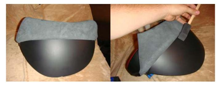
7. Paint a stripe of cement along the centerline of the hood from front to back. Pull the leather over the back center of the gauge hood and glue it down. Clip the leather into place as indicated by the single blue clip in the picture below. Work each side of the hood and add more clips as indicated below. You may find the leather bunches together. This is okay because you will pull the material under the hood and stretch out the leather for a smooth finish.
