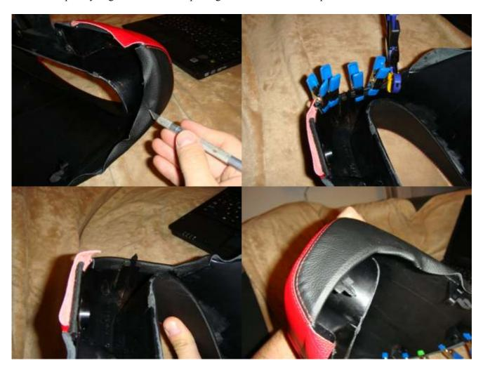
9. Check your work and look for any loose leather flaps on the rear edge. There isn't a lot of excess material to go around. This is where the painter's tape comes in handy. Glue any loose flaps down and use the tape to hold the flaps in place while the glue dries. Painters tape is strong enough to hold the leather down, but comes up without leaving any residue on the leather.
