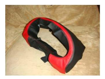
2. Start by stretching the leather and getting it into position on the hood. Be careful with any clamps. Squeeze too tight and the plastic will crack. It's a strong plastic but also brittle and the hood costs over \$100 to replace with a new one.
