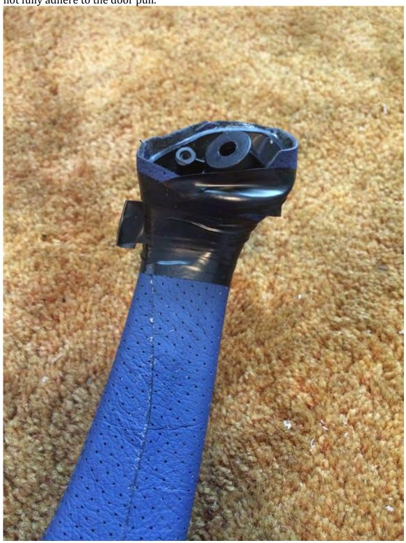
10) At this point the door pull should pretty much be done. Some light trimming may be necessary, but overall it should fit. Much of the excess you should be able to tuck underneath.
