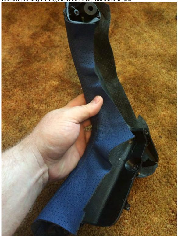
9) While the adhesive is drying, wrap tightly some electrical tape around the top of the pull. This will cause enough pressure to keep the leather in contact with the door pull as the adhesive cures. Give this plenty of time. If you don't then the leather will
