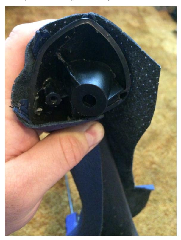
3) Once you have the seam and ridge aligned start by using a clamp at the bottom to secure the leather to the door pull.
