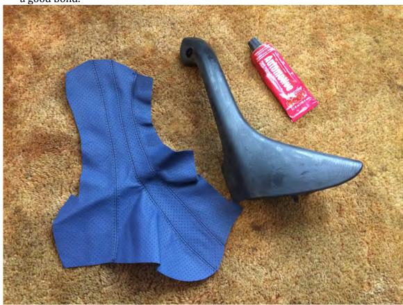
2) The key of the entire install is to start by aligning the seam flush (below) with the ridge just above the primary upper screw hole. There will likely be a bit of overlap on either side of this point that is not a problem.
